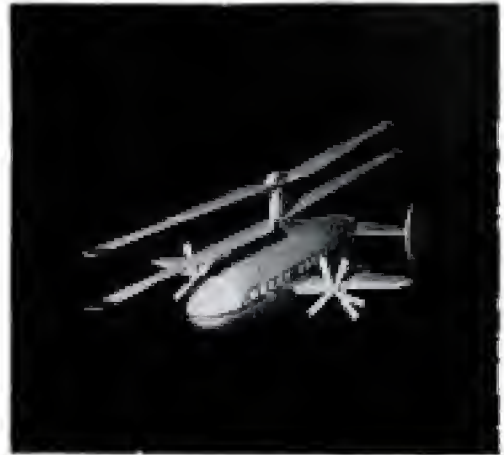
Rotor blades of Gyraliner model telescope inward to reduce drag in forward flight
